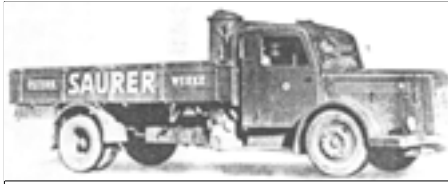
Illustration 2: Saurer BT 4500 with producer gas generator. 84 A Saurer truck similar to this type allegedly was used for mass murder in Kulmhof/Chelmno – not with producer gas, but incredibly with its exhaust gas. 85
